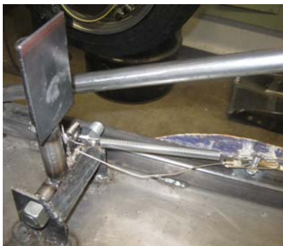
Throttle cable attached to the pedal
